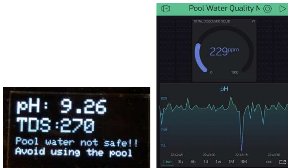
Figure 3. Data visualization both OLED display and Blynk application
