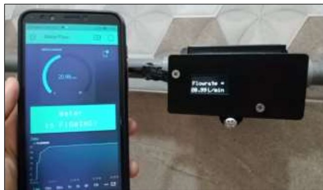
Figure 7. Results from the receiver (Blynk apps) and transmitters (device)
